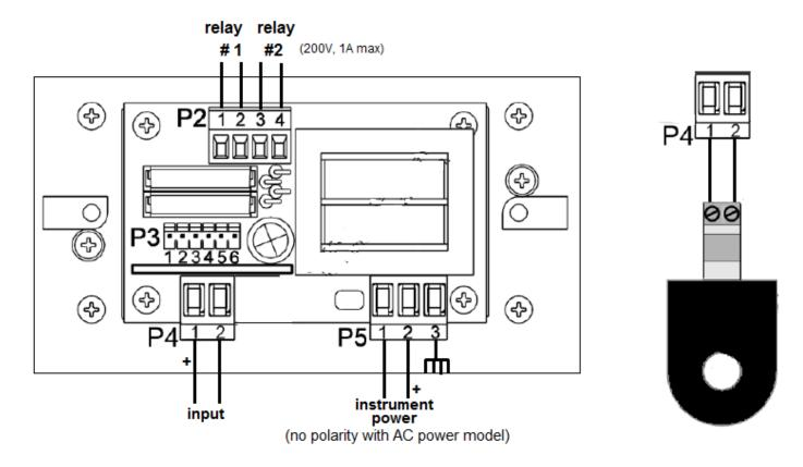
P3 pin header is a secondary function that duplicates the front panel control buttons. 1 = COMMON 2 = TARE 3 = SETPOINT/RESET 4 = PEAK 5 = VALLEY 6 = MENU Short or jumper temporarily function (pin 2 through 6) to pin 1.
